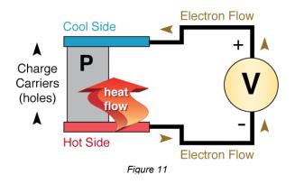
In thermoelectric power generation, 'P' pellets are also employed. *Figure 11* shows a basic configuration. Note how the flow of electrons goes in a direction *opposite* to that of hole flow.
