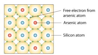
Figure 3: Arsenic dopant adds free electrons to the crystalline lattice, making it more electrically conductive, creating 'N' material.
