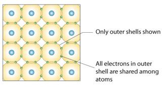
Figure 2: With four electrons in the outer shell, silicon atoms form a stable crystalline lattice by sharing electrons with each other.
