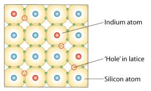
Figure 4: Indium dopant leaves "holes" in the crystalline lattice, making it more electrically conductive while creating 'P' material.
