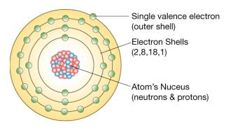
Figure 1: Structure of the copper atom
