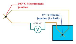
Figure 9: Thermocouple using 0° C reference junction.
