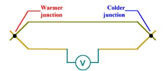
Figure 8: Breaking the circuit, allows for the measurement of the Seebeck voltage which is produced.
