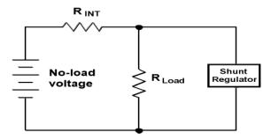
tub to the overflow drain, it begins to siphon off water to keep the tub from overflowing. With the shunt regulator, if the TEG is producing power that would normally take the load voltage beyond the desired operating point, the regulator will begin to conduct. By drawing additional current, it can drop more voltage across the internal resistance of the TEG module.
