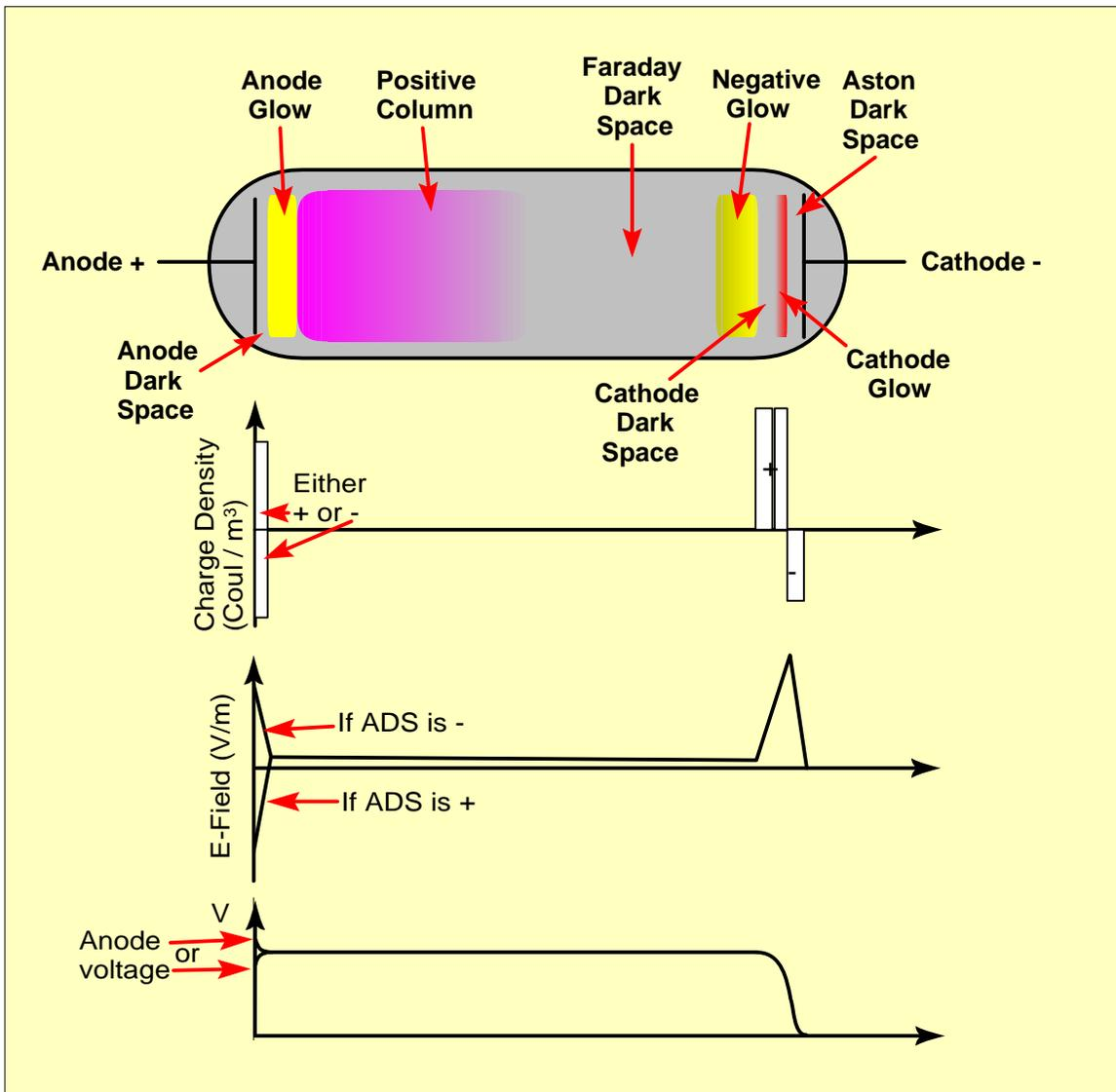
**Figure 1 (Top).** The physical appearance of an archetypical gas discharge. (Below) Charge density, *E*-field, and Voltage distributions within the tube. The bottom three plots will be discussed in parts two and three of this paper.
