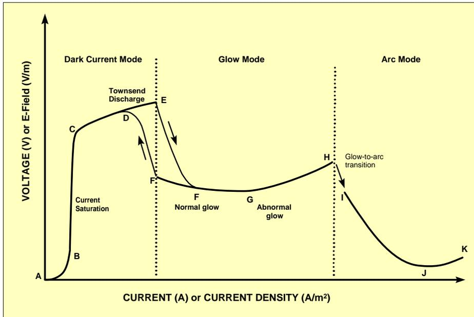
**Figure 4** A typical static, plasma discharge, volt-ampere plot. It is obviously highly nonlinear. A similar plot for a linear resistor would be a straight line, starting at the origin (point A) and rising upward toward the right. The angle of the line would be determined by the ohmic value of the resistor. The slope of a line from the origin to any point on the curve =  $V_p/I = R_p$  of the plasma.
