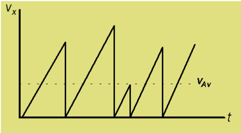
**Figure 6. A constant strength electric field (force per unit charge) creates a constant acceleration. The velocity of each carrier will increase linearly with time until it collides with another particle. This produces an average velocity value,  $v_{Av}$  that is proportional to the applied field.**
