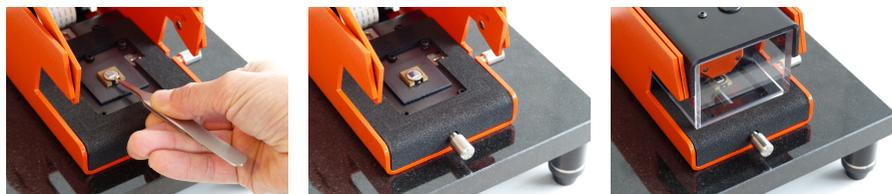
**Figure 3-10: Placing a sample.** Left: Use the tweezers to place the sample onto the sample stage. Center: Sample is held in place by the magnet of the sample stage. Right: NaioAFM closed for measurement.
