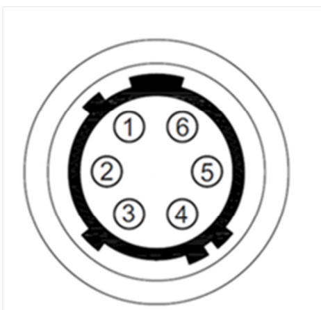
Figure 4 The gas cell heater connector employs a Hirose 6-pin connector. The pin out is given on the right.
