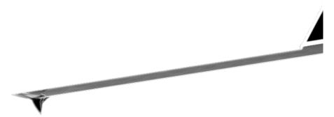
Figure 18-1: Cantilever. 228 μm long micro-fabricated silicon cantilever with integrated tip.
