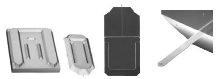
**Figure 3-1: Cantilever.** (Left) Alignment system. (Center) Cantilever chip viewed from the top. (Right) Cantilever, 450 µm long. 50 µm wide with integrated tip.
