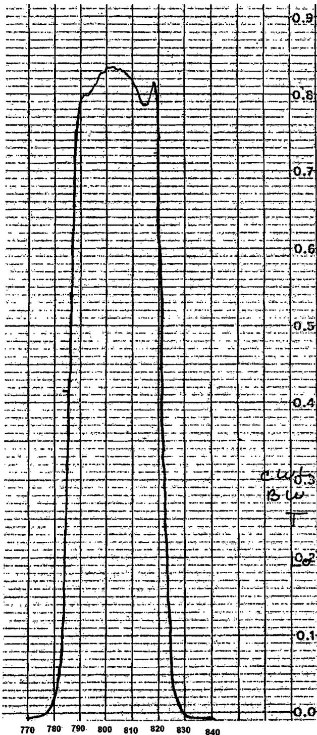
**Interference filter:** Diameter 50mm. The transmission characteristics of the filter are shown in Figure 3C-1. We are mostly interested in the Rubidium D lines at 780nm and 795 nm. The transmission peak of the interference filter may be "tuned" to shorter wavelengths by rotation about the vertical axis. If  $\lambda_0$  is the peak wavelength then when the filter is tilted at an angle  $\theta$  the new peak wave length will be given by,
