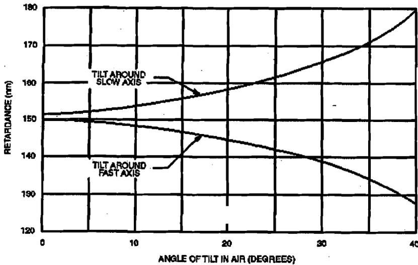
Figure 3C-3 Tilt Tuning of Quarter Wave Plate.
