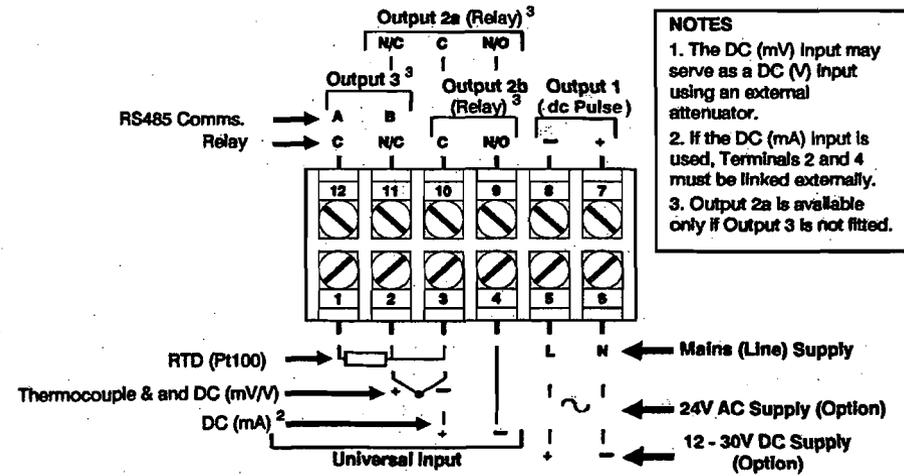
**FIGURE 2-1** Rear Terminal Connections
