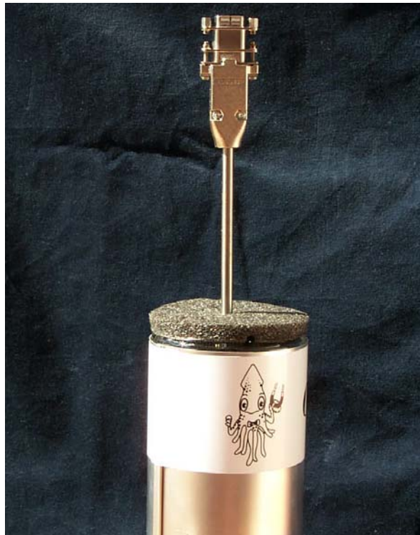
Figure 2-3 Mr. SQUID ® inserted into liquid nitrogen dewar.
