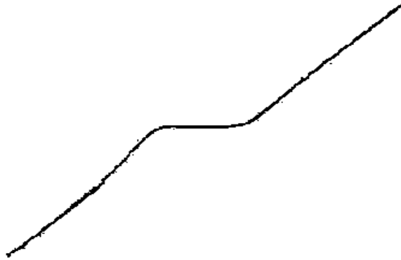
Figure 3-3 Typical Mr. SQUID ® V-I characteristic.
