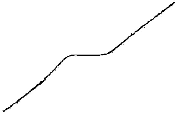
Figure 4-3 A typical Mr. SQUID ® V-I characteristic.
