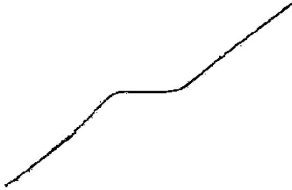
Figure 5-4 A typical Mr. SQUID ® V-I characteristic.
