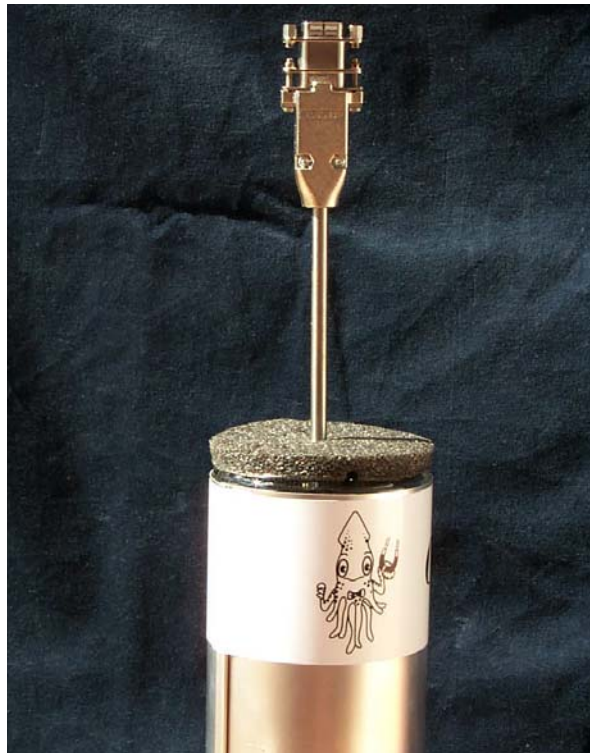
Figure 2-3 Mr. SQUID ® inserted into liquid nitrogen dewar.
