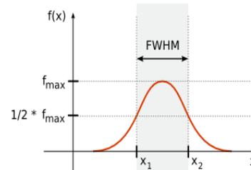
The full width at half maximum (FWHM) is a parameter commonly used to describe the width of a "bump" on a curve or function. It is given by the distance between points on the curve at which the function reaches half its maximum value.
