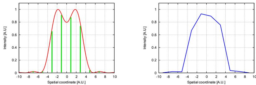
The Nyquist criterion states that, in order to prevent undesired aliasing, one must sample a signal at a rate equal to at least twice its bandwidth.
