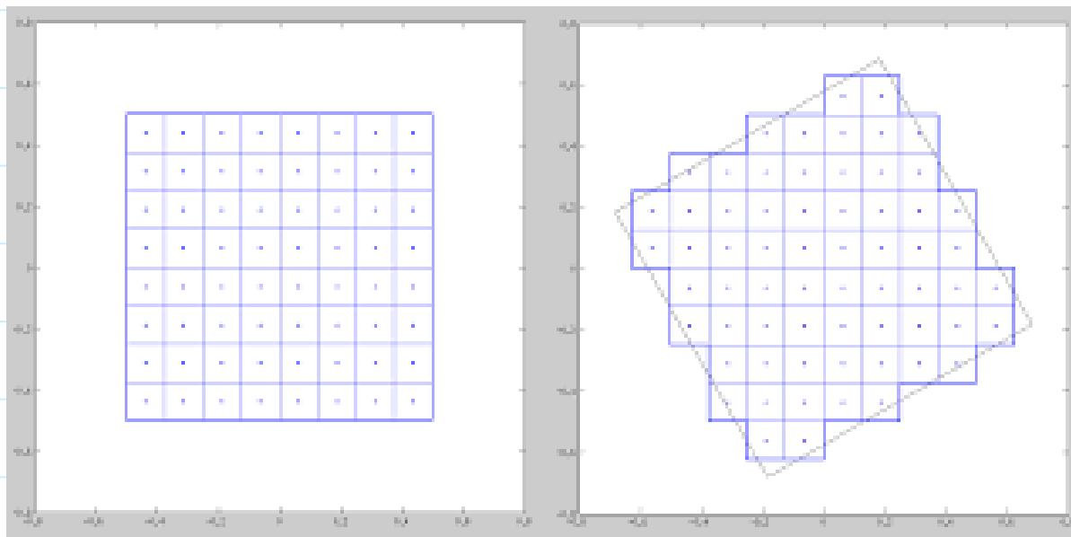
Note the "staircasing" that arises (except for a square domain). Alternative: finite element meshes
