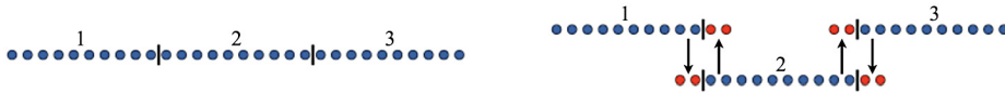
Fig. 5. One dimensional line segmentation analogous to the multidimensional parallel decomposition of a patch.
