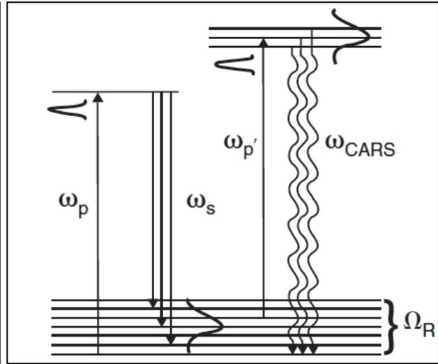
$$\omega_{AS} = \omega_L + \omega_{vib} = \omega_L + (\omega_L - \omega_s)$$
