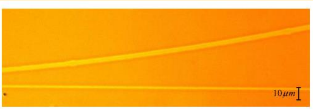
5. Top-view microscope image of parts of bus and ring waveguides, directly written in a thin layer of As_2S_3 .
