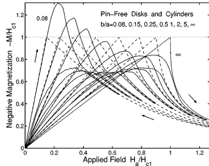
FIG. 3. Irreversible magnetization curves  $-M(H_a)$  of pin-free circular disks and cylinders with aspect ratios  $b/a=0.08, 0.15, 0.25, 0.5, 1, 2, 5,$  and  $\infty$  in axial field (solid lines). In these type-II superconductors the irreversibility is due to a purely geometric edge barrier for flux penetration. The dashed curves are the reversible magnetization curves of the corresponding ellipsoid defined by Eqs. (1), (4), and (5).
