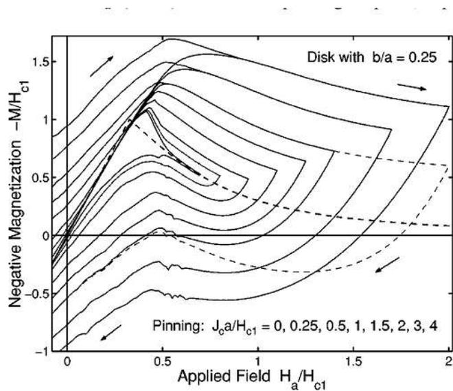
FIG. 4. Magnetization curves of a thick disk with aspect ratio  $b/a=0.25$  for various degrees of volume pinning,  $J_c=0, 0.25, 0.5, 1, 1.5, 2, 3, 4$  in units  $H_{c1}/a$ , and for various sweep amplitudes. The inner loop belongs to the pin-free disk ( $J_c=0$ ), the outer loop to strongest pinning. Also shown is the reversible magnetization curve of the corresponding ellipsoid (dashed curve). All loops are symmetric,  $M(-H_a)=-M(H_a)$ .
