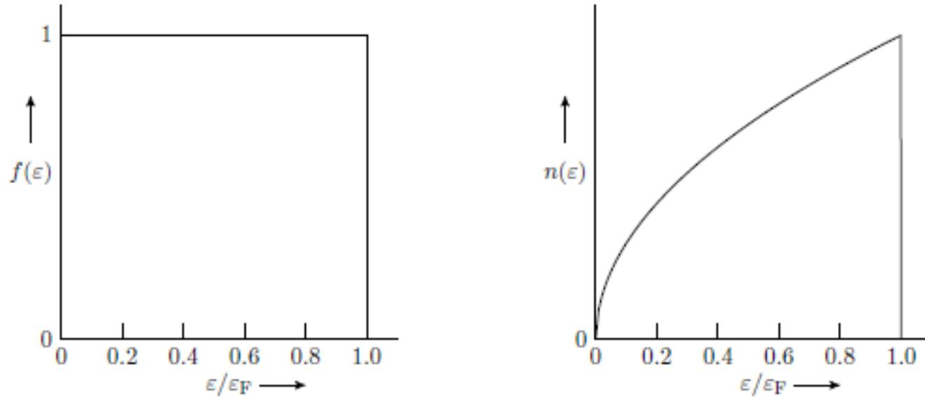
Figure 2: The Fermi-Dirac mean occupation number  $f(\varepsilon)$  and energy distribution  $n(\varepsilon)$  for a non-relativistic fermion gas at zero temperature:  $T = 0$  K. The energy is expressed in units of the Fermi energy  $\varepsilon_F$ .
