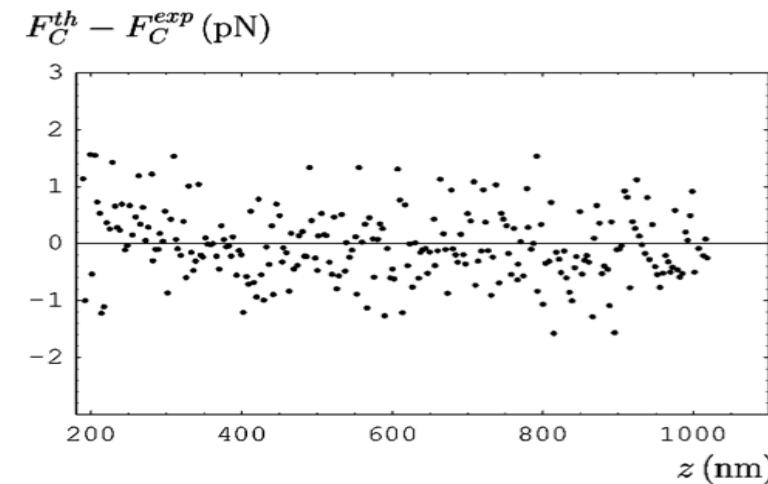
FIG. 10. Difference of the theoretical and experimental Casimir forces between the sphere and plate versus separation obtained from the static measurement.
