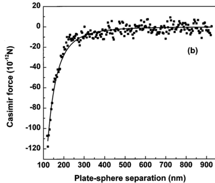
FIG. 3. (a) A typical force curve as a function of the distance moved by the plate; (b) the measured Casimir force corresponding to (a) as a function of sphere-plate surface separation. The solid line is the theoretical Casimir force from Eq. (4).
