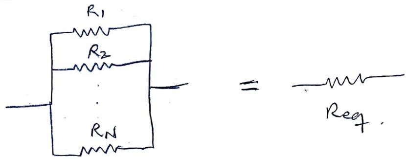
$$\text{con } R_{eq} = \left( \frac{1}{R_1} + \frac{1}{R_2} + \dots + \frac{1}{R_N} \right)^{-1}$$
