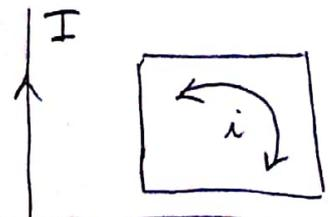
$$\Rightarrow i = \frac{\mu_0 \dot{I} l}{2\pi R} \ln\left(\frac{D+l}{D}\right) = -\frac{\mu_0 l \alpha}{2\pi} \ln\left(\frac{D+l}{D}\right) \cdot \frac{I(t)}{R} < 0$$
