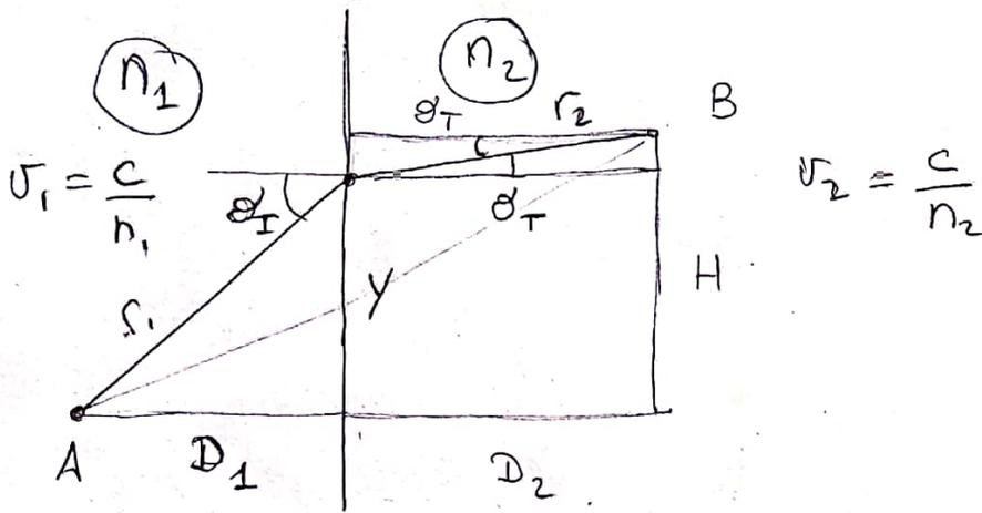
$$T = \frac{r_1}{v_1} + \frac{r_2}{v_2}, \quad r_1 = \sqrt{D_1^2 + y^2}$$
