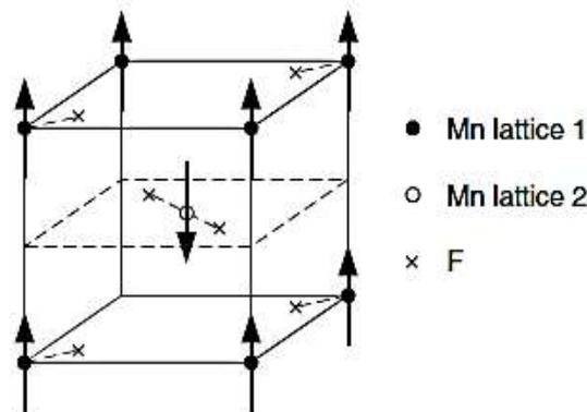
Fig. 6.7. Structure of the anti-ferromagnetic insulator MnF<sub>2</sub>
