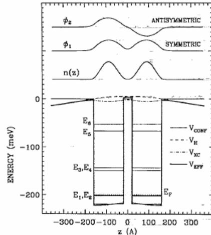
FIG. 1. The typical double quantum well structure ( $N_s = 10^{11} \text{ cm}^{-2}$ ) with the self-consistent local-density-approximation calculated energy levels and wave functions for the symmetric-antisymmetric levels. The bare ( $V_{\text{conf}}$ ), Hartree ( $V_H$ ), and exchange-correlation ( $V_{\text{xc}}$ ) contributions to the effective potential ( $V_{\text{eff}}$ ) are shown. (The SAS gap  $\Delta_{\text{SAS}} = |E_2 - E_1|$ .)
