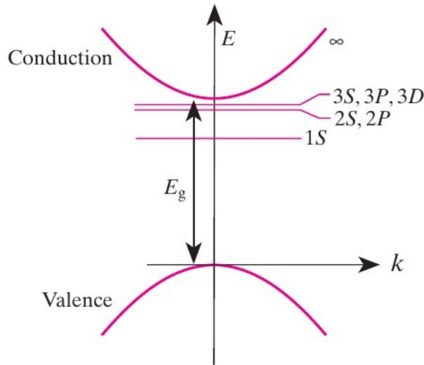
**Fig. 4.1.** Schematic diagram of the  $n=1$ , 2, and 3 bound states of a shallow donor electron near a nondegenerate and parabolic conduction band (corresponding to  $n = \infty$ ).  $E_g$  is the bandgap
