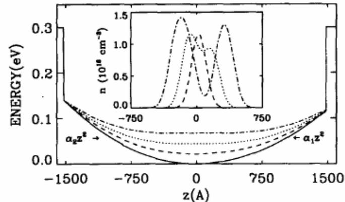
Fig. 1. Model bare potential of the asymmetric parabolic well (solid line), and calculated self-consistent potentials with an in-plane magnetic field of  $B = 5.8 T$ , for  $N_s = 2.4$  (dash line),  $4.7$  (dotted line), and  $7.5 \times 10^{10} \text{ cm}^{-2}$  (dash-dot line); inset: corresponding calculated self-consistent densities.
