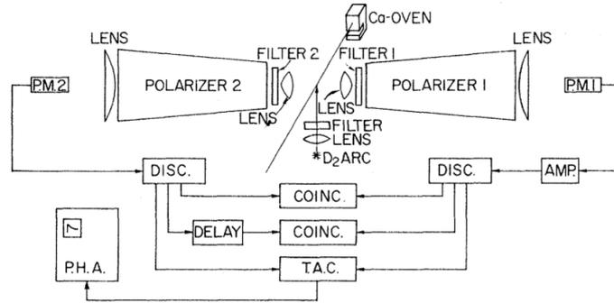
**FIG. 1.** Schematic diagram of apparatus and associated electronics. Scalers (not shown) monitored the outputs of the discriminators and coincidence circuits during each 100-sec count period. The contents of the scalars and the experimental configuration were recorded on paper tape and analyzed on an IBM 1620-II computer.
