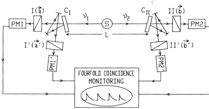
FIG. 2. Timing experiment with optical switches. Each switching device ( $C_I, C_{II}$ ) is followed by two polarizers in two different orientations. Each combination is equivalent to a polarizer switched fast between two orientations.
