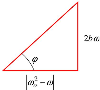
$$\begin{aligned} \operatorname{sen} \varphi &= \frac{2b\omega}{\left[ (\omega_0^2 - \omega^2)^2 + (2b\omega)^2 \right]^{1/2}} \\ \operatorname{cos} \varphi &= \frac{(\omega_0^2 - \omega^2)}{\left[ (\omega_0^2 - \omega^2)^2 + (2b\omega)^2 \right]^{1/2}} \end{aligned}$$
