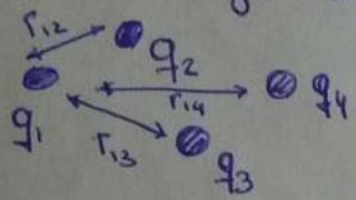
$$\vec{F}_1 = \frac{q_1}{4\pi\epsilon_0} \left[ \frac{q_2}{r_{12}^2} \frac{(\vec{r}_1 - \vec{r}_2)}{|\vec{r}_1 - \vec{r}_2|} + \frac{q_3}{r_{13}^2} \frac{(\vec{r}_1 - \vec{r}_3)}{|\vec{r}_1 - \vec{r}_3|} + \frac{q_4}{r_{14}^2} \frac{(\vec{r}_1 - \vec{r}_4)}{|\vec{r}_1 - \vec{r}_4|} \right]$$
