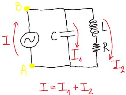
$$\begin{aligned} V_0 &= 220 \text{V} \\ f &= 50 \text{Hz} \\ \omega &= 2\pi f \end{aligned}$$
