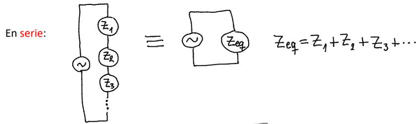
$V_o = V_{10} + V_{20} + V_{30} + \dots$
